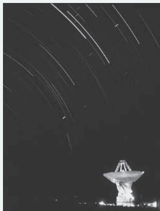
FIGURE 1.8 The search for extraterrestrial life is being carried out with radio antennas like the one pictured here. A radio antenna is an example of a system with position controls.
